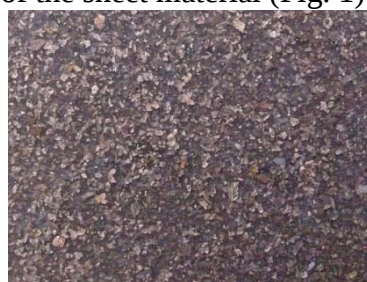
Fig. 1. The material is obtained as a result of extrusion of metallized granules
