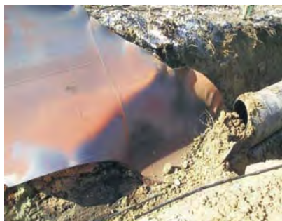
Fig. 5. An example of typically destroyed pipeline
