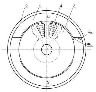
Fig. 1. PMDC motor with radial magnets.
