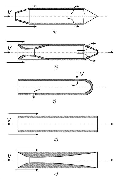
Fig.1. The schematic diagrams of the aerodynamic chambers: a) deceleration chamber with the longitudinal flow-around and diverging entry; b) deceleration chamber with the longitudinal flow-around and converging entry; c) transverse flow-around chamber; d) cylindrical chamber with a constant cross-section; e) critical speed chamber
