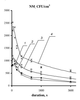
Fig. 1. NM dependence of B.cereus bacteria during process duration: Ar/US (1),  $O_2$ /US (2), He/US (3) and  $CO_2$ /US (4). Initial data:  $NM_0 = 8 \cdot 10^2$  CFU/cm<sup>3</sup>. Conditions:  $T = 298 \pm 1$  K
