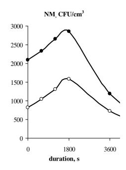
Fig. 2. NM change of natural water during US treatment. Initial data:  $NM_{01} = 820$  CFU/cm<sup>3</sup> (1) and  $NM_{02} = 2090$  CFU/cm<sup>3</sup> (2). Conditions:  $T = 298 \pm 1$  K
