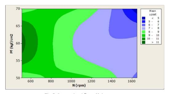
Fig. 7. Contour plot of  $P_f$  vs N for mean upset
