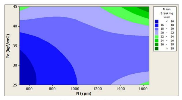
Fig. 10. Contour Plot of mean breaking load
