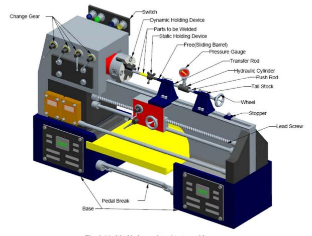
Fig. 1. Modified lathe machine friction welding setup
