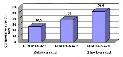
Fig. 1. Results of compressive strength test after heat treatment of fine-grained concretes (PC:S:BS=1:1.2:0.69)
