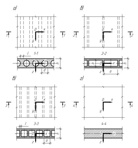
Fig.1. Actual (a, b, c) and calculated (d) Section monolithic slabs with tubular inserts
