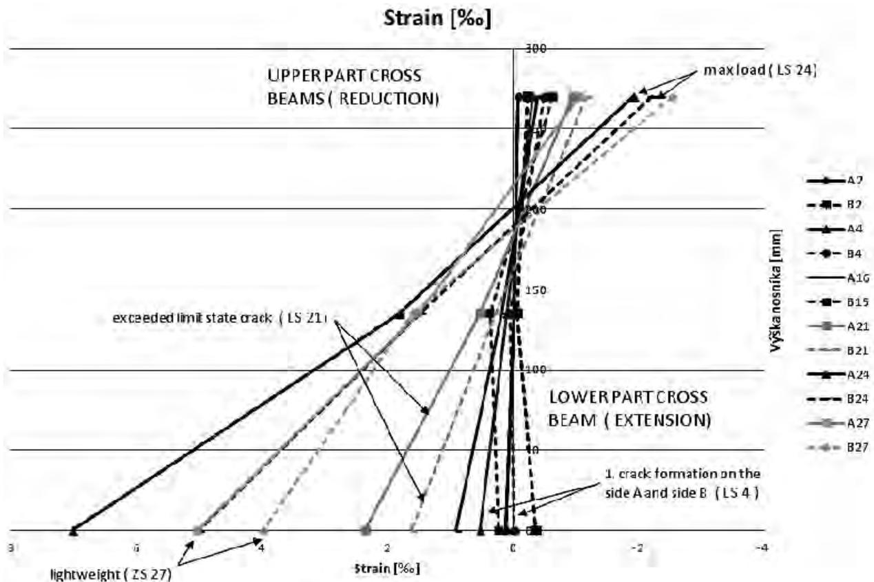
Fig. 6. Graphical representation of strain during the height of the beam
