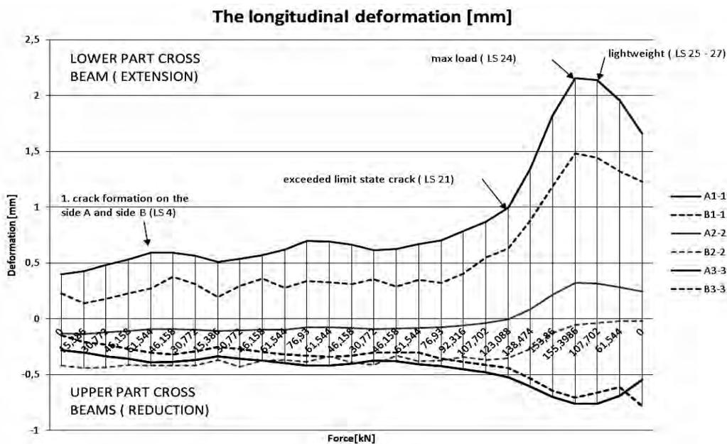
Fig. 4. Graph of longitudinal deformation and strength during loading
