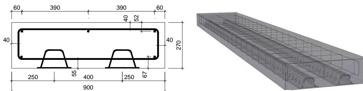
Fig. 1. Size and shape of beam N1
