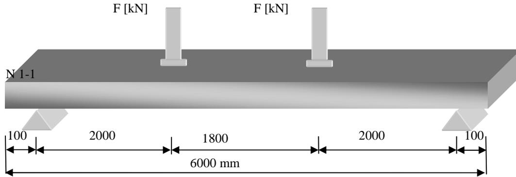
Fig. 2. Static scheme supported beam
