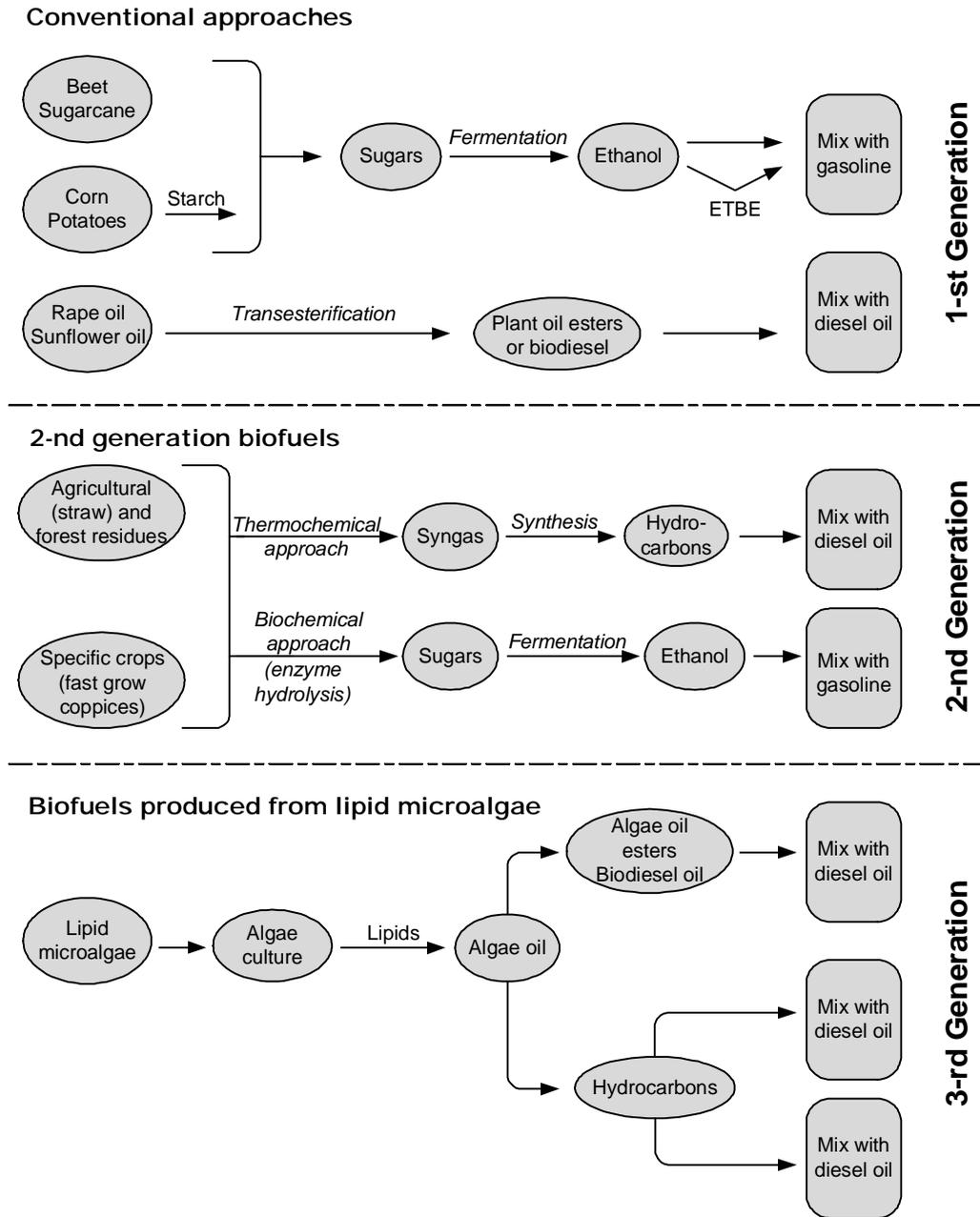
**Fig. 2.** Development of technologies for biofuels production [2, 15]
