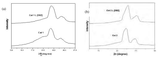
**Fig. 4.** X-ray diffraction of copolymers synthesized by catalysts 1 (a) and catalyst 2 (b) with low (L) amount of DEZ and without DEZ
