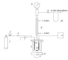
**Fig. 3.** Autoclave plant for cyclohexane oxidation: oxygen cylinder (1); reducer (2); valves (3, 7, 8); control equipment
