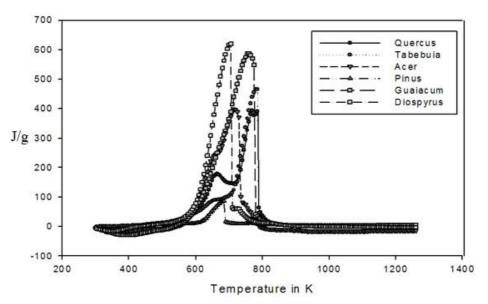
Fig. 3. Overlay of DTA curves for all seven species of wood, showing the multiple energetic events discussed below. Curves show the normalized heat flow for the samples
