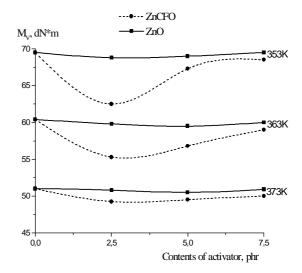
**Fig. 4.** Rheological properties of the modeling rubber mixes on the basis of isoprene rubber with a various type and contents of sulfur vulcanization activators
