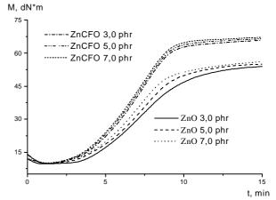
Fig. 8. Cure curves of metaloxide vulcanization process of modeling elastomeric compositions on the basis of chloroprene rubber at 428K with various type and contents of vulcanization agents
