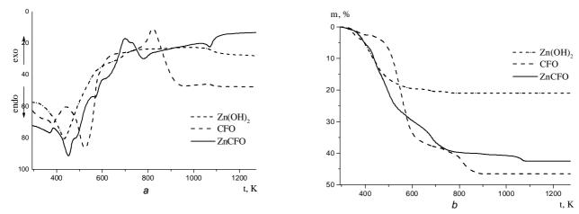
Fig. 2. Results of derivatographic researches of Zn(OH)<sub>2</sub>, CFO and ZnCFO: DTA curves (a) and TG curves (b)
