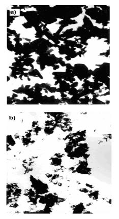
Fig. 1. EM micrographs of the ZnO (a) and ZnCFO (b) particles (increase in 10000 times)
