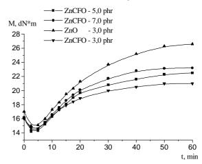
**Fig. 9**. Vulcanization kinetics of modeling elastomeric compositions on the basis of butyl rubber of resin vulcanization at 433 K with ZnO or ZnCFO
