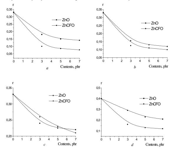
Fig. 11. Dependence of particles size of heterophase of modeling compositions on the basis of various rubbers with different vulcanization systems from the ZnO or ZnCFO contents: nitrile-butadiene rubber of sulfur vulcanization (a); nitrile-butadiene rubber of thiuram vulcanization (b); nitrile-butadiene rubber of peroxide vulcanization (c) and chloroprene rubber of metaloxide vulcanization (d)
