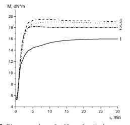
**Fig. 5.** Rheometer data of sulfur vulcanization process of modeling elastomeric compositions on the basis of isoprene rubber at 428 K with ZnCFO as the activator:
