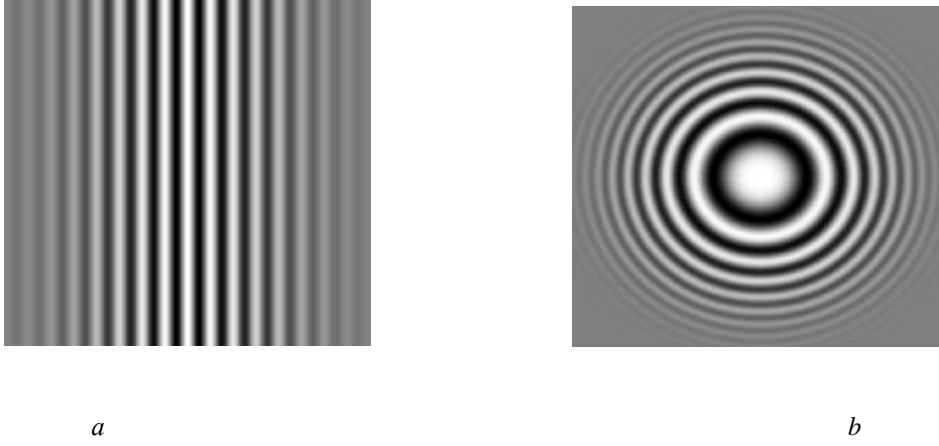
Fig.5. The interferograms of simulated surfaces: a – tilted, b – spherical
