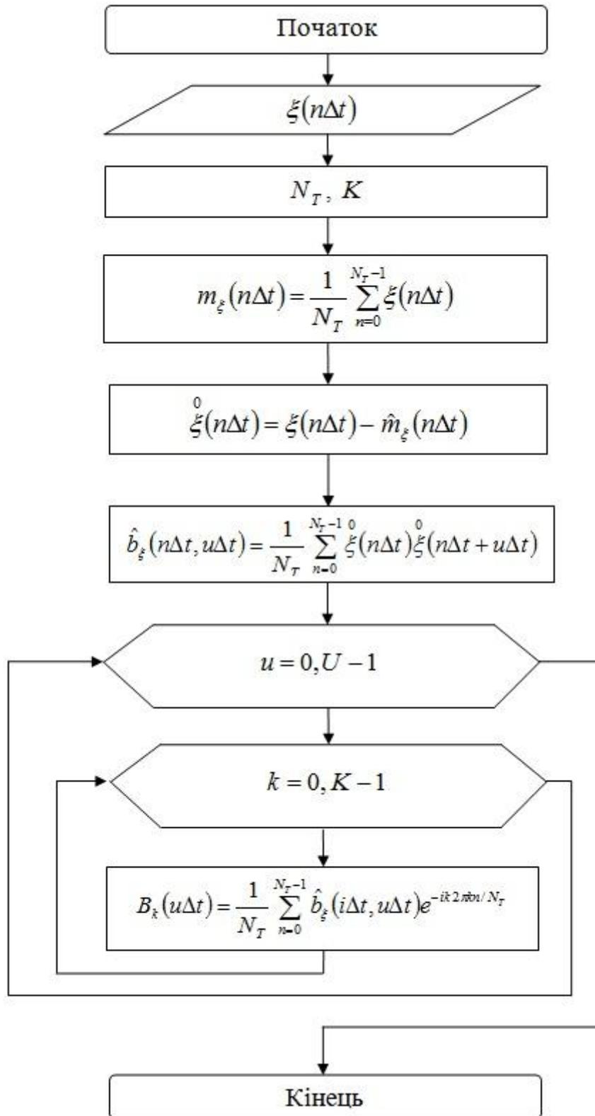
Figure 1. Block diagram EGS component method processing
