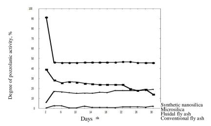
Fig. 2. Degree of pozzolanic activity of the mineral additives
