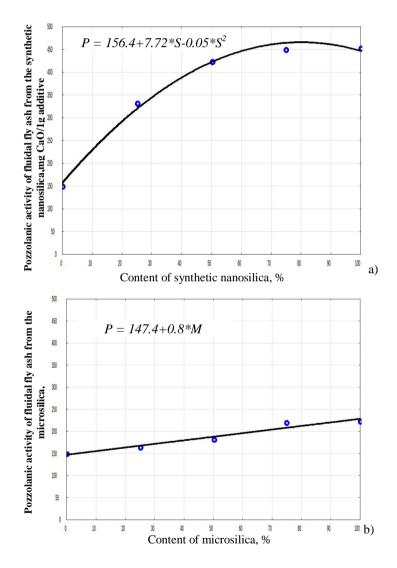
**Fig. 3.** Models of regression function for the dependence of pozzolanic activity on content of synthetic nanosilica (a) and microsilica (b). For the formula: P – pozzolanic activity; S – content of synthetic nanosilica; M – content of microsilica
