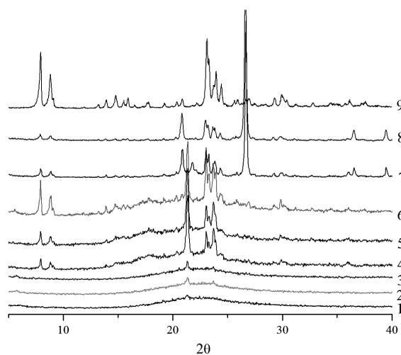
**Fig. 2.** Samples diffractogram at different hydrothermal temperature and time: 353 K, 11 h (1); 353 K, 24 h (2); 353 K, 48 h (3); 393 K, 11 h (4); 393 K, 24 h (5); 393 K, 48 h (6); 448 K, 24 h (7) and 448 K, 48 h (8). Reference sample of ZSM-5 (9) is given for the comparison
