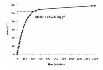
Fig. 9. Effect of contact time on the adsorption of Cr(VI) ion onto chitosan beads
