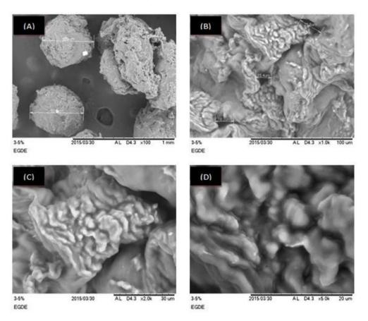
**Fig. 2.** SEM micrographs of chitosan beads under the optimum conditions (5 % TPP, 5 % EGDE, 3 h immersion time). Magnification of  $100 \times (a)$ ;  $1000 \times (b)$ ;  $2000 \times (c)$  and  $5000 \times (d)$
