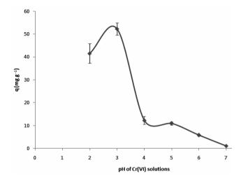
Fig. 8. Effect of pH on the adsorption of Cr(VI) onto chitosan beads
