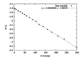
Fig. 13. Graph of the exponential function concentration of Cr(VI) adsorbed on the chitosan beads per time t
