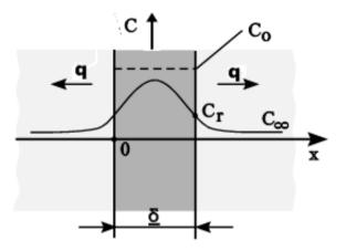
**Fig. 1.** A schematic drawing of the mass transfer from lamina:  $C_0$  – concentration in lamina (in the internal cell volume) at reference time;  $C_r$  – concentration on the edge;  $C_{\mathfrak{X}}$  – concentration in the solution flow; q – mass flow from the surface; d – thickness of lamina (leaf)
