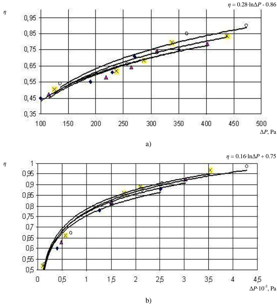
**Fig. 7.** Dependence of entrapping efficiency on hydraulic resistance of drop catcher (a) and mist eliminator (b):  $\square$  –  $F/G = 0$ ;  $\blacklozenge$  –  $F/G = 0.05$ ;  $\blacktriangle$  –  $F/G = 0.10$ ;  $\times$  –  $F/G = 0.15$ ;  $\circ$  –  $F/G = 0.20$
