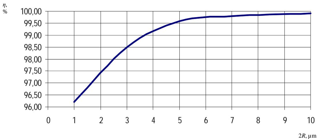
**Fig. 4.** Entrapping efficiency at the 2<sup>nd</sup> stage of separation (filter-coalescer)
