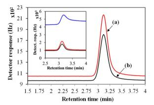
**Fig. 1.** Typical chromatograms of SF<sub>6</sub> standard (159.82 nmol·mol<sup>-1</sup>) obtained with CON (a) and CAR (b) make-up gas. The chromatogram of SF<sub>6</sub> standard obtained without make-up gas (uppermost line in inset) is also included for comparison only
