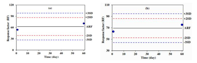
**Fig. 3**. The chart of control limit for the measurement of SF<sub>6</sub> standard at concentration of 11.87 nmol·mol<sup>-1</sup> using CON (a) and CAR (b) make-up gas. For interpretation of the references to color in the figure, the reader is referred to the web version of the article
