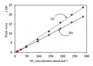
**Fig. 4.** Linear response of nine SF<sub>6</sub> standards ranging from 6.65 to 284.79 nmol·mol<sup>-1</sup> for CON (a) and CAR (b) make-up gas
