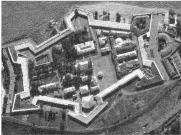
Fig. 5. A restored by inverse filter image with NAE = 9,2% and NMSE = 1,2%.
