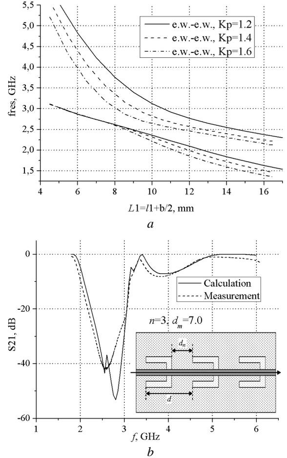
Fig. 4. The characteristics of the microstrip resonator with nonsymmetric  $\Pi$ -shaped slot, Fig 1a: (a) eigenfrequency spectrum, and (b) insertion losses of 3-cells periodic structure. The resonator parameters (in mm): substrate  $h=1.0$ ,  $\epsilon_r=9.8$ , the microstrip line width  $w=1.0$  (characteristic impedance  $Z_0=50$  Ohm), screen dimensions  $b_1=9.0, b_2=5.0, A=24.0$ , slot resonator dimensions:  $a=8.0, b=8.0, s_1=0.5, s_2=0.75$ .
