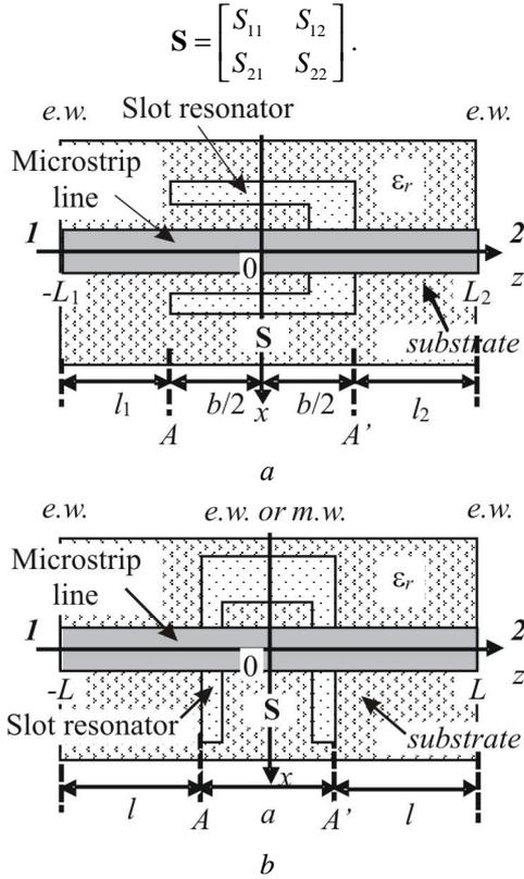
Fig. 1. *P*-shaped slot resonator in the microstrip line ground plane: (a) non-symmetric and (b) symmetric discontinuity.
