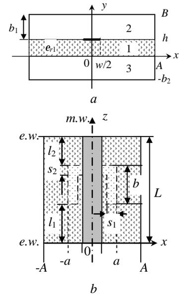
Fig. 2. Topology of the boundary problem: cross section (a) and top view (b) of the microstrip resonator with non-symmetrically located *P*-shaped slot discontinuity in the ground plane.
