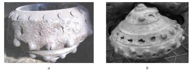
Fig. 2. Appearance of the destroyed roller cone drill bit 269,9 VS-PV with the most loaded crowns of cones: a – the fall out and destruction of the rock-destructive part of hard-alloyed cutters and the rolled cones crown; b – falling out of the hard-alloyed cutters of cone
