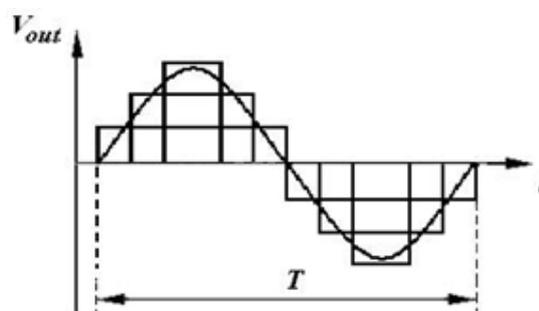
Fig. 1. Forming the output ac voltage at multilevel dc voltage commutation.
