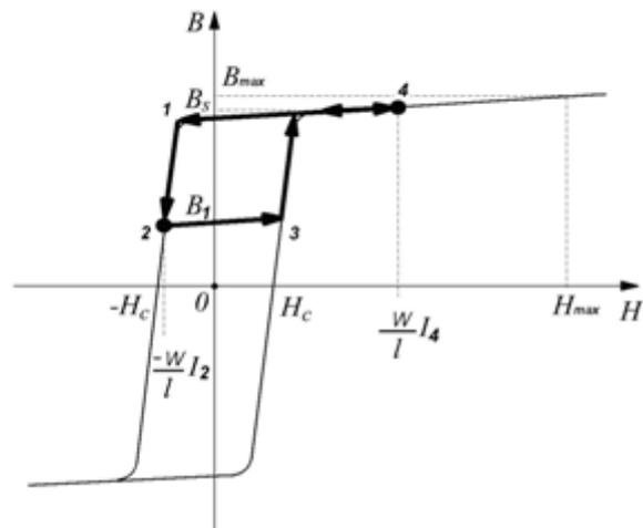
Fig. 3. B-H characteristic (hysteresis loop) of MagAmp core material.
