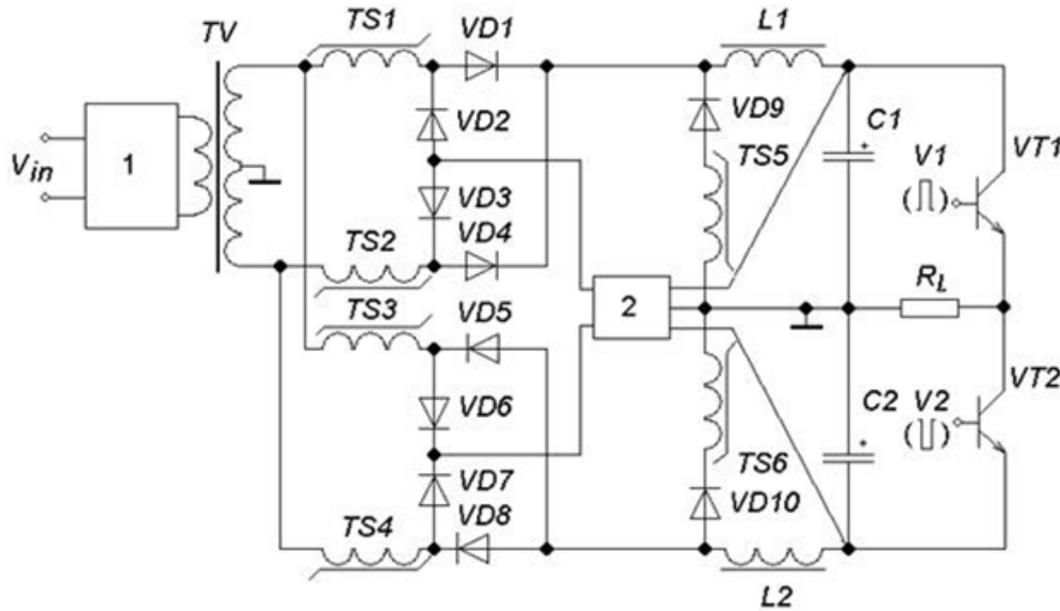
Fig. 6. Proposed circuit diagram of MagAmp Power Inverter (1 – uncontrolled transistor inverter; 2 – control circuit).
