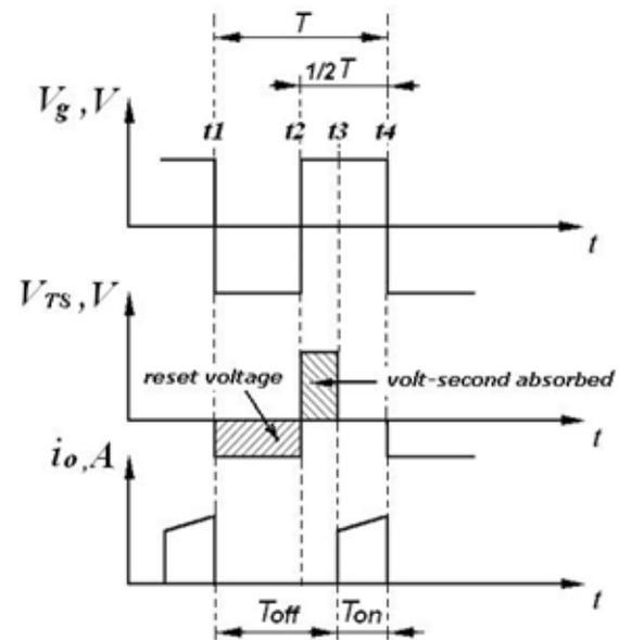
Fig. 4. Ideal MagAmp waveforms:  $V_g$  is secondary winding transformer voltage,  $V_{MS}$  is MagAmp switch voltage;  $i_o$  is MagAmp switch output current.
