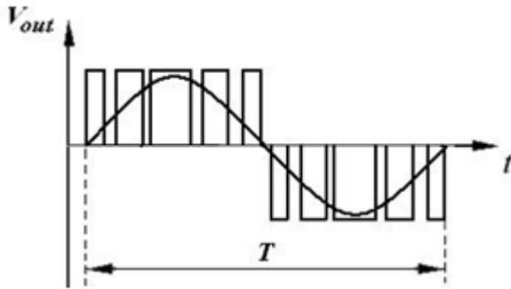
Fig. 2. Forming the output ac voltage by pulse-width modulation of high-frequency power switches.
