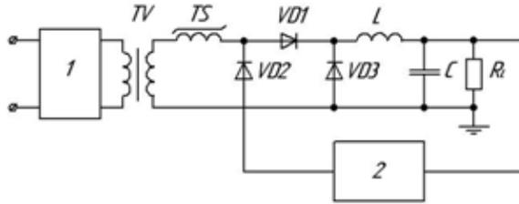
Fig. 5. Functional diagram of the voltage regulator based on the MagAmp switch (1 is an unregulated high-frequency transistor inverter; 2 is a control circuit).
