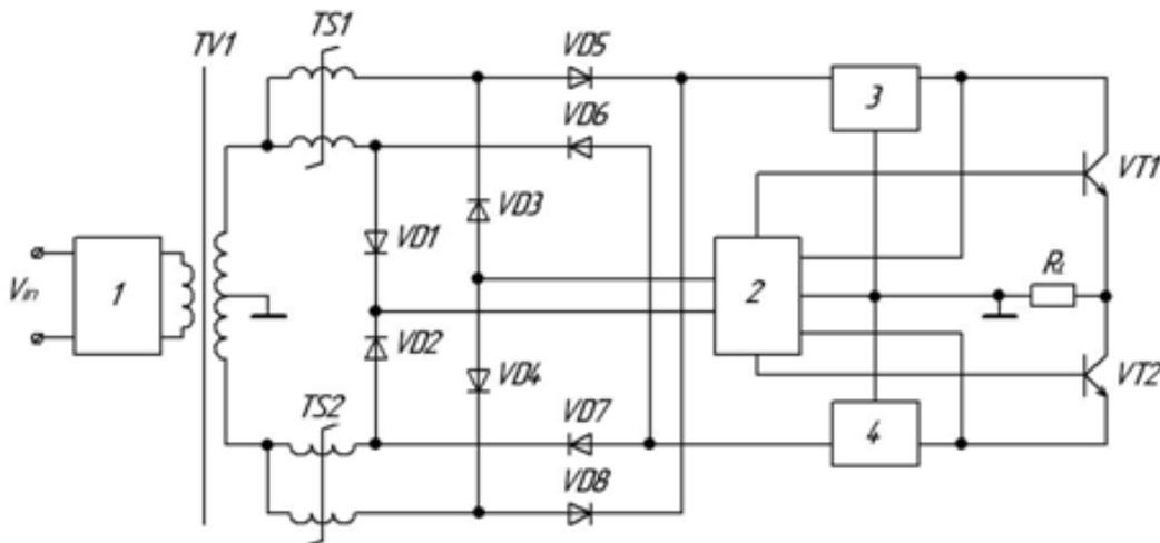
Fig. 7. Improved functional diagram of proposed high-frequency MagAmp inverter (1 – uncontrolled transistor inverter; 2 – control circuit; 3, 4 – output filters).
