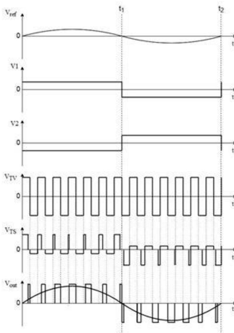
Fig. 8. Theoretical waveforms of MagAmp inverter.
