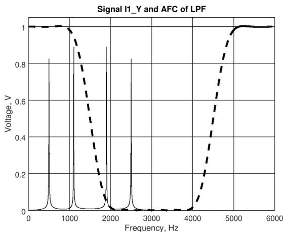
Fig. 4. Internal signal  $I1\_Y$  in the frequency domain and amplitude-frequency characteristic of the LPF (dashed curve).
