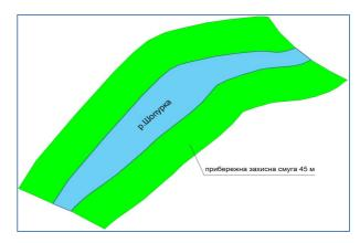
Fig. 5. Diagram of the protective riparian zone along the river Shopurka (part) according to formula (1)
