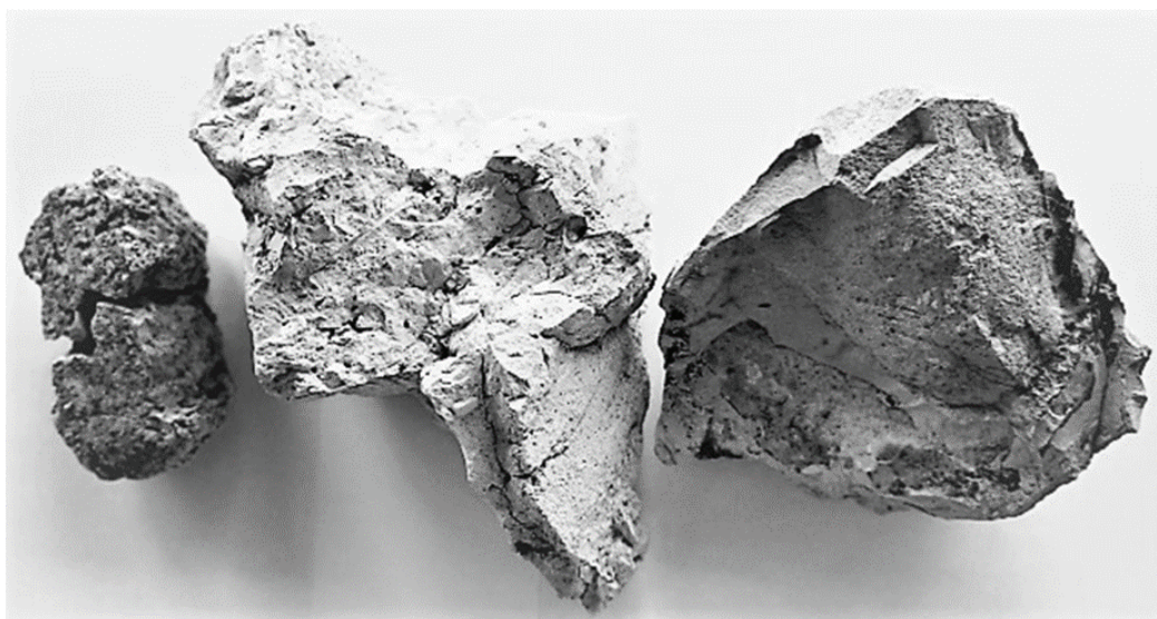
Fig. 3. Sequence of materials and materials from the retort: writing chalk, partially modified chalk with horseshoe replicas (b), microcrystalline carbonate (c).
