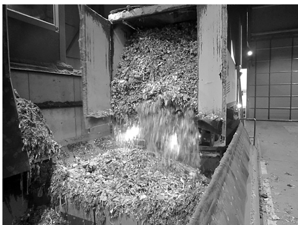
Fig. 6. Uploading of typical RDF to be used as fuel for CFB gasification at FW's gasifier
