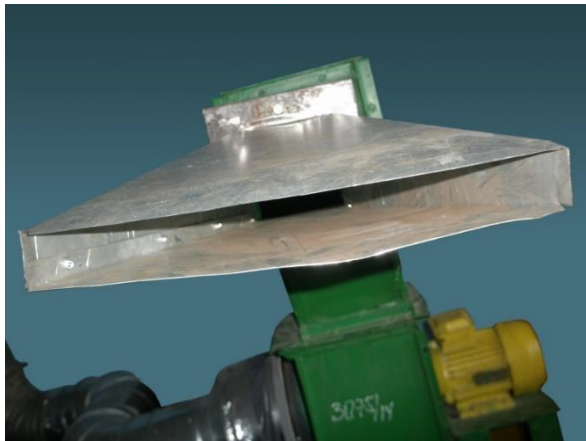
Fig. 5. Full-scale experimental samples of adapters from the end of 10 \times 10 cm at the end of adapter 3 \times 30 cm
