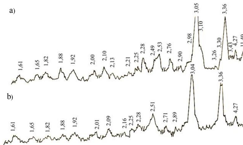
Fig. 4. X-ray patterns of hydrated BPLP:AA<sub>L</sub> mixtures with different ratios (w/w): 20:80 (a) and 10:90 (b). Setting conditions: 2 days, 413 K, 60 MPa
