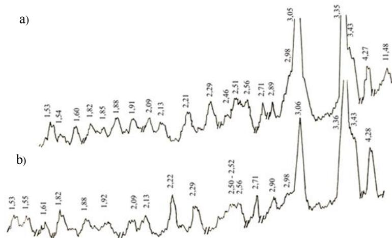
**Fig. 6.** X-ray patterns of hydrated BPLP:AA<sub>K</sub> mixtures with different ratios (w/w): 20:80 (a) and 10:90 (b). Setting conditions: 2 days, 413 K, 60 MPa
