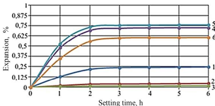
**Fig. 7.** Kinetics of expansion for BPLP:AA<sub>L</sub> mixtures with different ratios (w/w): 10:90 (1, 2, 3) and 20:80 (4, 5, 6). Setting conditions:  $T = 348 \text{ K}$ ,  $P = 30 \text{ MPa}$  (1, 4);  $T = 378 \text{ K}$ ,  $P = 40 \text{ MPa}$  (2, 5);  $T = 413 \text{ K}$ ,  $P = 60 \text{ MPa}$  (3, 6)
