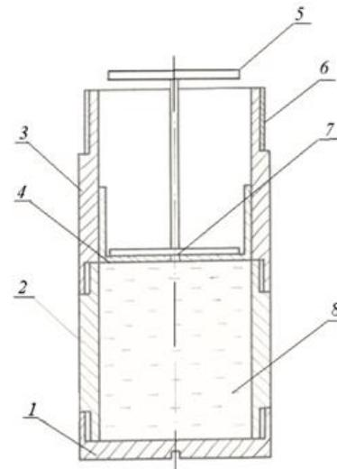
**Fig. 1.** Consistometer attachment to determine the expansion of plugging materials: 1 – removable bottom of the glass; 2, 3 – elements of the glass body; 4 – separating piston; 5 – coil; 6 – connecting thread; 7 – hole; 8 – plugging solution
