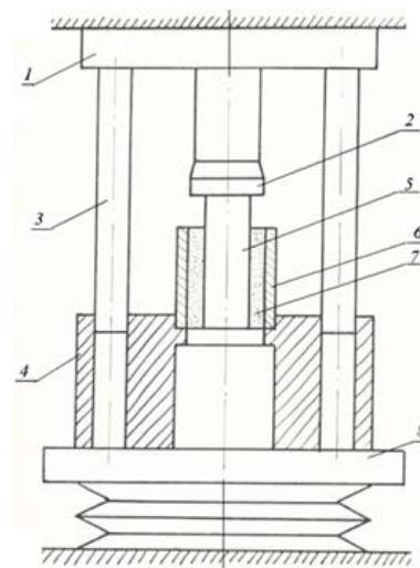
**Fig. 2.** PSU press attachment to determine the adhesion of cement stone with metal: 1 – pressure plate; 2 – cylinder; 3 – the rod-clamp; 4 – housing; 5 – metal rod; 6 – cylindrical shape; 7 – cement stone; 8 – movable plate of the hydraulic press PSU-10
