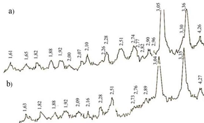
Fig. 5. X-ray patterns of hydrated BPLP:AA<sub>L</sub> mixtures with different ratios (w/w): 20:80 (a) and 10:90 (b). Setting conditions: 14 days, 373 K, 40 MPa
