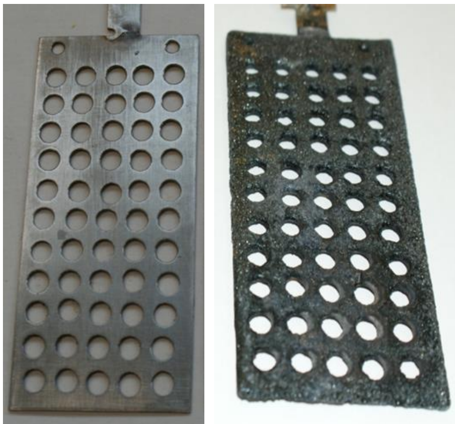
Fig. 3. Basis for the manufacture of bench anodes and the finished anode
