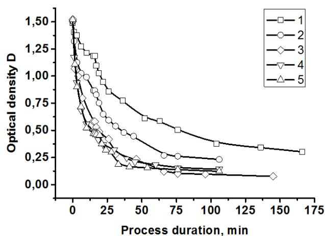
Fig. 7. Kinetic curves of MB oxidation on  $CoFe_2O_4/SiO_2/CuO$  with different amount of the catalyst in reactive medium in terms of CuO: 1 –  $3 \cdot 10^{-5}$  mol; 2 –  $6 \cdot 10^{-5}$  mol; 3 –  $9 \cdot 10^{-5}$  mol; 4 –  $1.2 \cdot 10^{-4}$  mol; 5 –  $1.5 \cdot 10^{-4}$  mol
