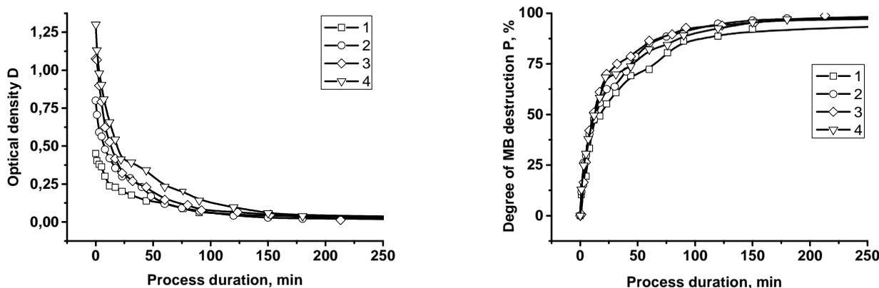
**Fig. 9.** Kinetic curves of MB oxidation on  $\text{CoFe}_2\text{O}_4/\text{SiO}_2/\text{CuO}$  with different concentration of MB in solution: 1 –  $2 \cdot 10^{-5}$  mol/L; 2 –  $3 \cdot 10^{-5}$  mol/L; 3 –  $4 \cdot 10^{-5}$  mol/L; 4 –  $5 \cdot 10^{-5}$  mol/L
