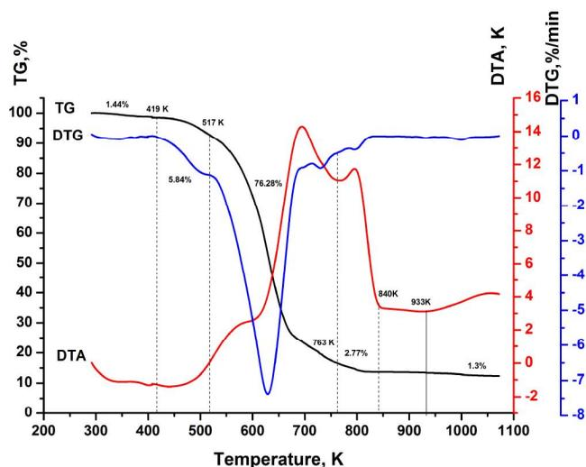
**Fig. 4.** Thermogram of the precipitate PMMA-Co(OH)<sub>2</sub>-Fe(OH)<sub>3</sub> after drying at 373 K
