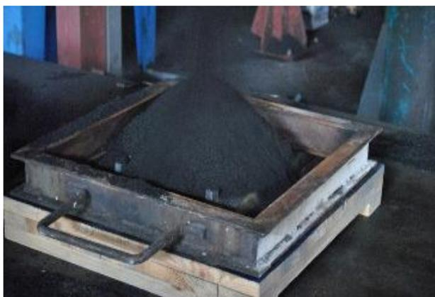
Fig. 1. Conditioned used molding mixture
