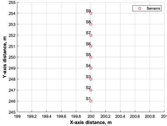
Fig. 5. Sensor placement with a distance of 1 m between them
