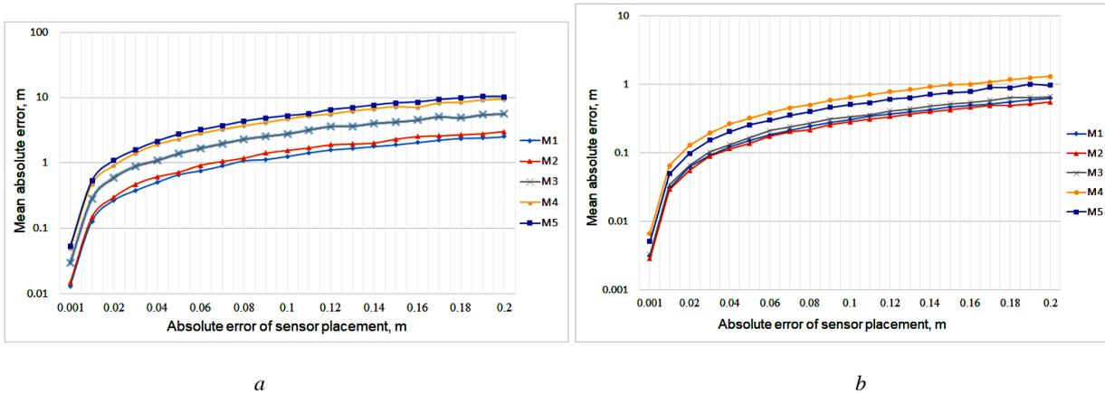
Fig. 3. Dependence of MAE on the absolute sensor detection error: *a* – X coordinate; *b* – Y coordinate
