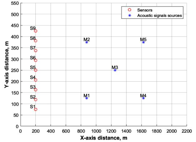
Fig. 2. Location of sensors and sound sources
