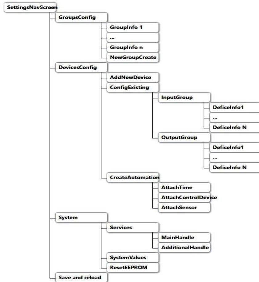
Fig. 4 The structural diagram of the settings menu
