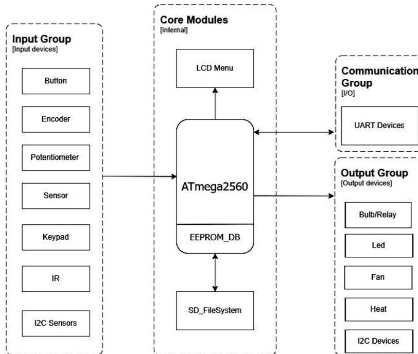
Fig. 1. Block diagram of services for connected devices
