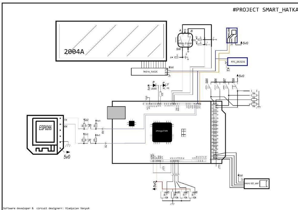
Fig. 7 The schematic of the connections to the main control unit
