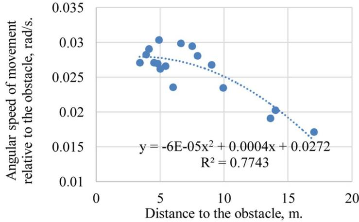
Fig. 6. Dependence of the change in angular velocity on the distance to the obstacle
