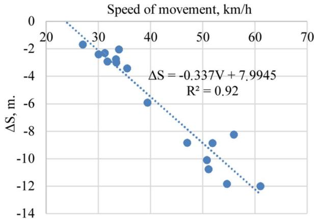
Fig. 4. The difference in the driver's subjective safety gap in the longitudinal direction of movement ( $S_d$ ) and braking distance ( $S_{br}$ )
