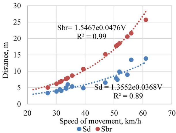
Fig. 2. Parameters of the driver's subjective safety gap in the longitudinal direction of movement ( $S_d$ ) and braking distance ( $S_{br}$ )
