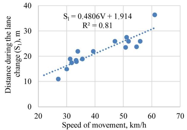
Fig. 3. Dependence of the distance during the lane change ( $S_1$ ) from the primary speed
