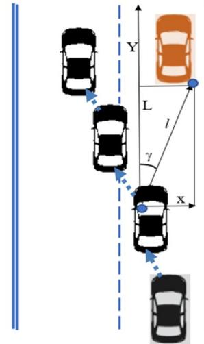
Fig. 5. Scheme of location of vehicles for determining the angular speed
