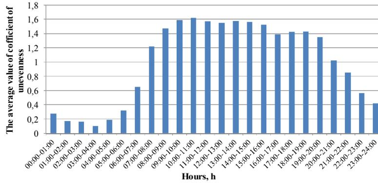
Fig. 1. The graph of changes in the coefficients of the unevenness of traffic flow by hours in the studied area
