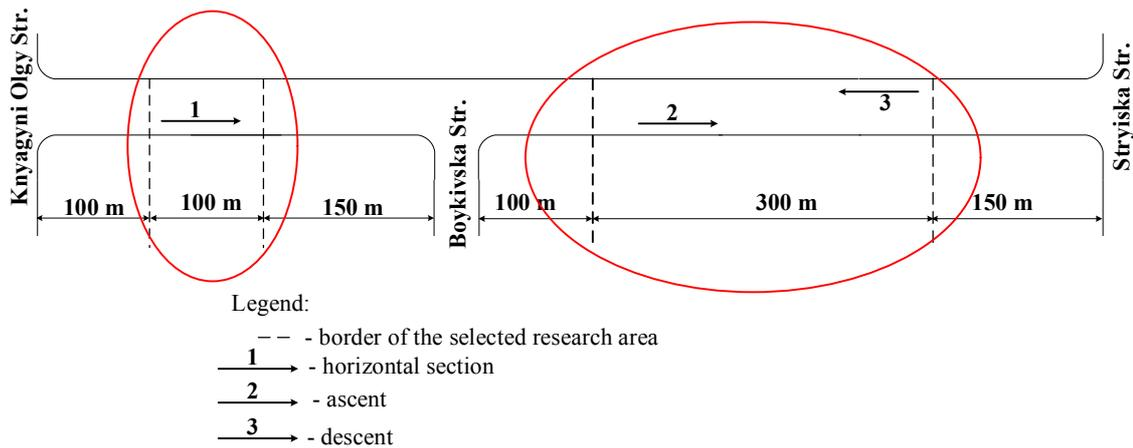
Fig. 4. The scheme of the section for determining the speed of the traffic flow
