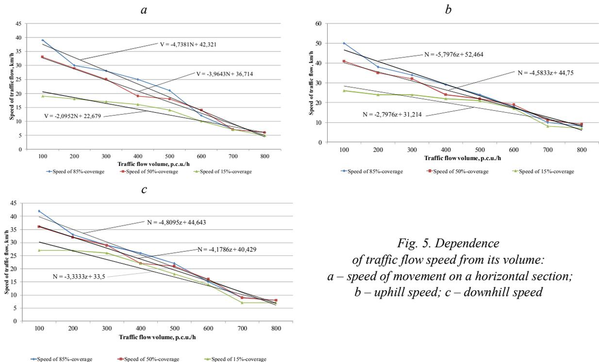
Fig. 5. Dependence of traffic flow speed from its volume: a – speed of movement on a horizontal section; b – uphill speed; c – downhill speed
