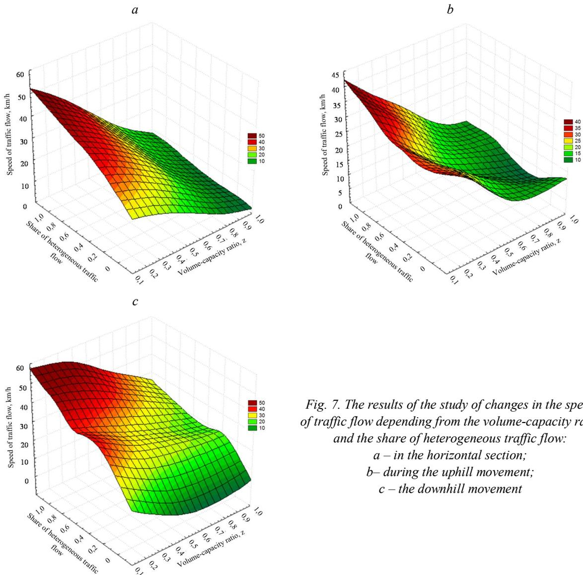
Fig. 7. The results of the study of changes in the speed of traffic flow depending from the volume-capacity ratio and the share of heterogeneous traffic flow:
