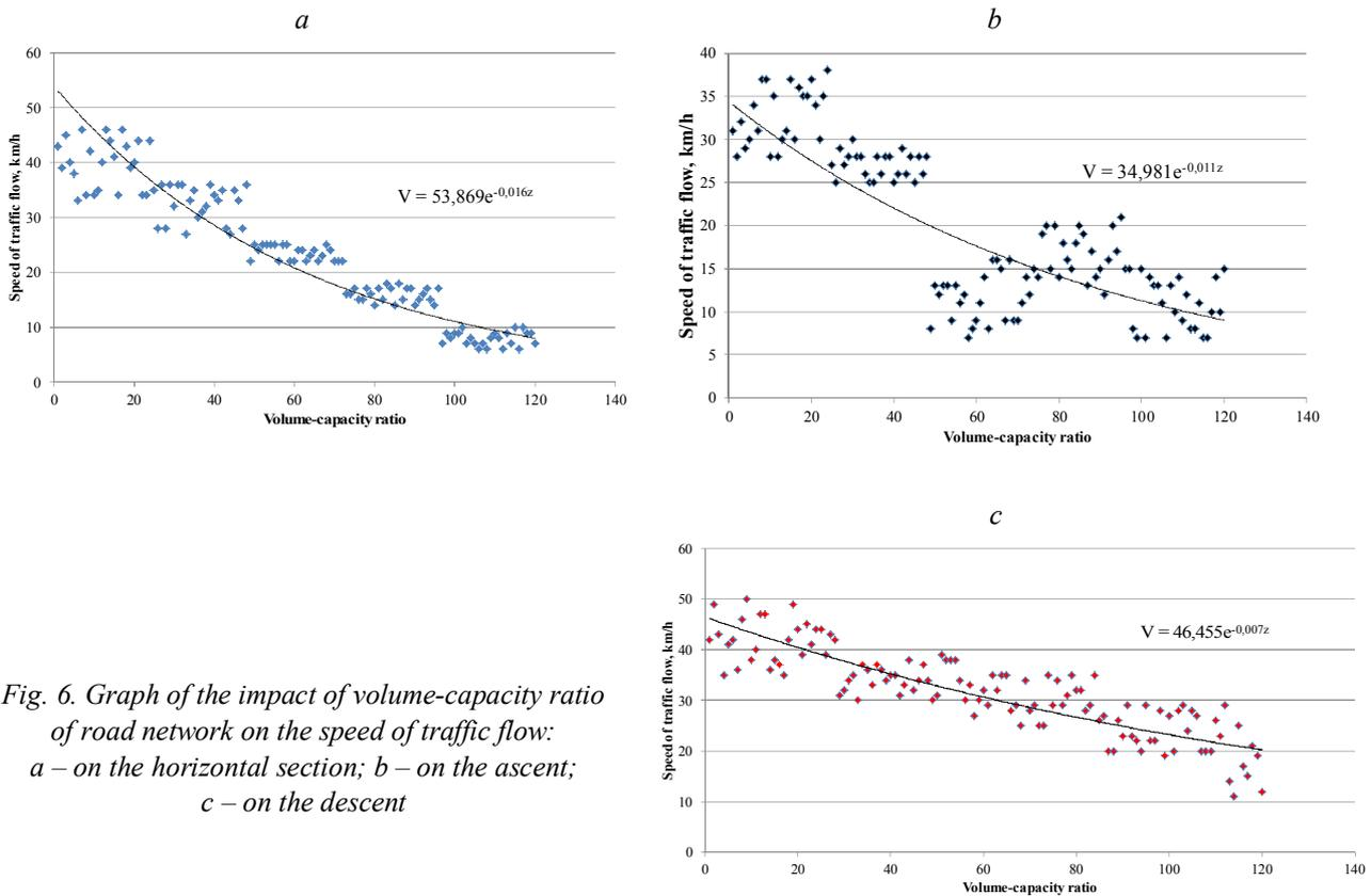
Fig. 6. Graph of the impact of volume-capacity ratio of road network on the speed of traffic flow: a – on the horizontal section; b – on the ascent; c – on the descent
