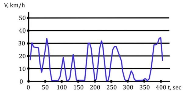
Fig. 4. Average urban driving cycle schedule based on experimental data for a 2.2 km route segment
