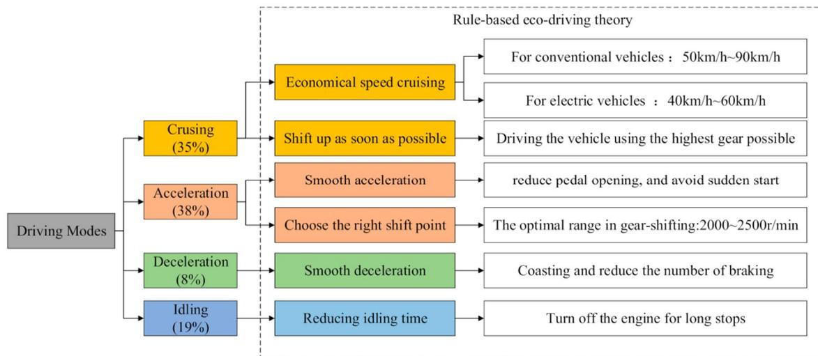
Fig. 1. Rule-based eco-driving theory in the main driving modes [5]
