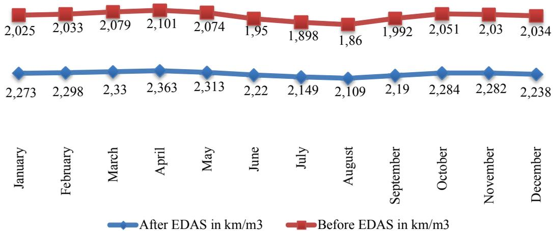
Fig. 2. Improvement in fuel efficiency through the use of an eco-drive system [1]
