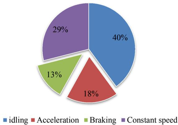
Fig. 3. The probability of a vehicle being in a certain driving mode [15]
