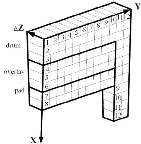
Fig. 1. Sector of the mesh model of the drum brake mechanism of the BOGDAN A091 bus
