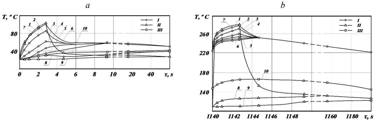
Fig. 2. Temperature change of elements of the front brake mechanism of the BOGDAN A091 bus during tests I: a – 1st cycle; b – 20th cycle; I – brake drum; II – overlay; III – side wall of the drum; 1 and 7 – friction surfaces; 2,3,4,5 and 6 – respectively at a distance of 1.5 mm, 4.5 mm, 10.5 mm, and 12 mm from the friction surface; 8 and 9 – respectively at a distance of 2.1 mm and 6.4 mm from the friction surface; 10 – the middle of the side wall of the drum
