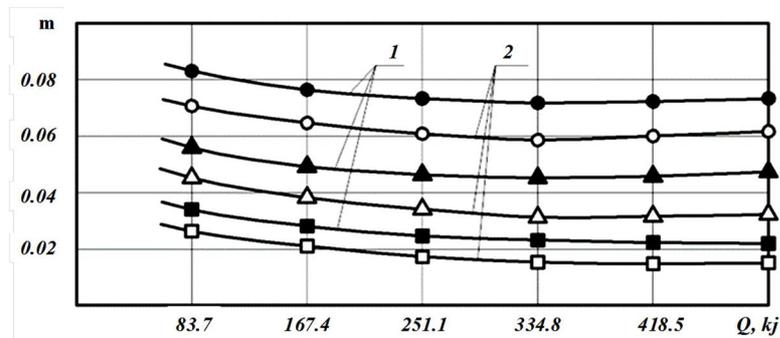
Fig. 4. Dependence of the heat flow distribution coefficient on  $h$  and  $Q$  during tests I: 1.  $\alpha = 34.8 \text{ W/m}^2\text{degr}$ ; 2.  $\alpha = 174 \text{ W/m}^2\text{degrees}$ ;
