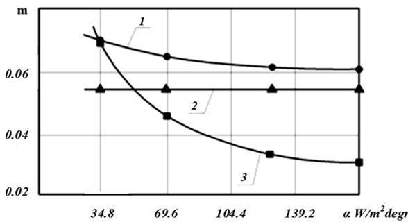
Fig. 3. Dependence of the coefficient of heat flow distribution on the heat transfer coefficient (test I,  $Q=251.2$  kJ):
