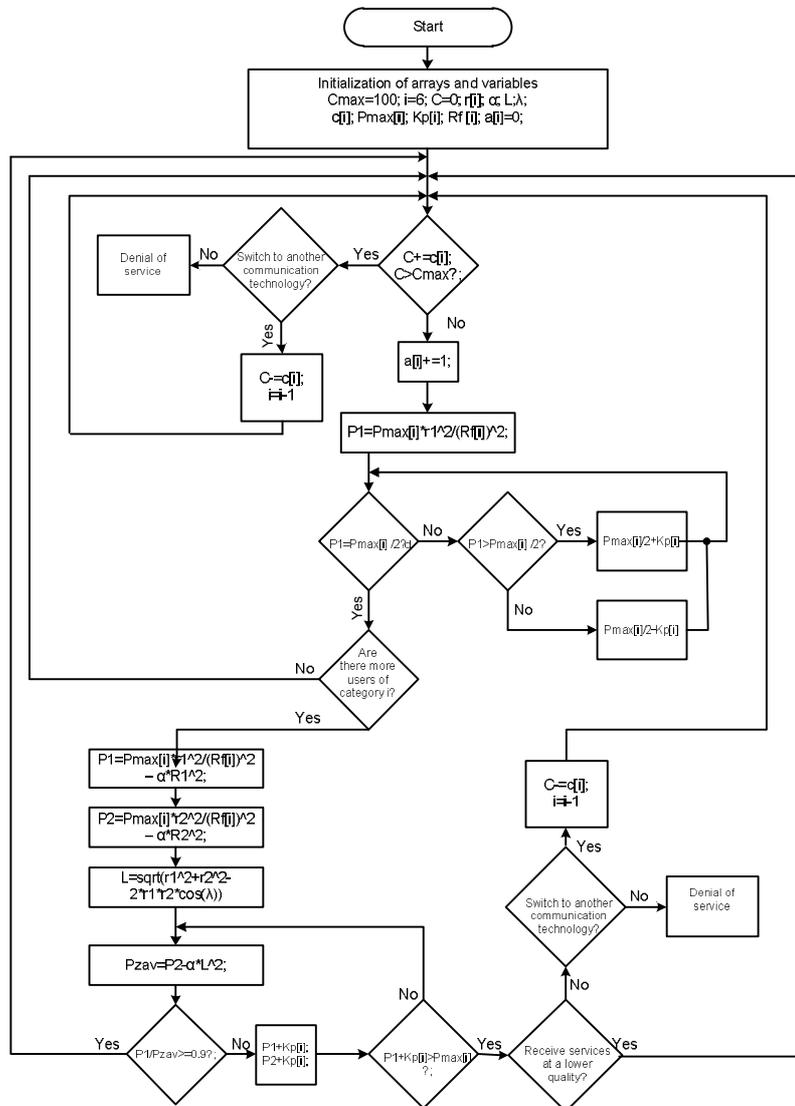
Fig. 13. Algorithm of the model for managing radio interfaces and physical resources of a femtocell
