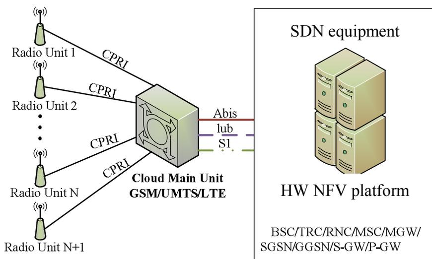
Fig. 2. Architecture of a software-defined heterogeneous mobile network
