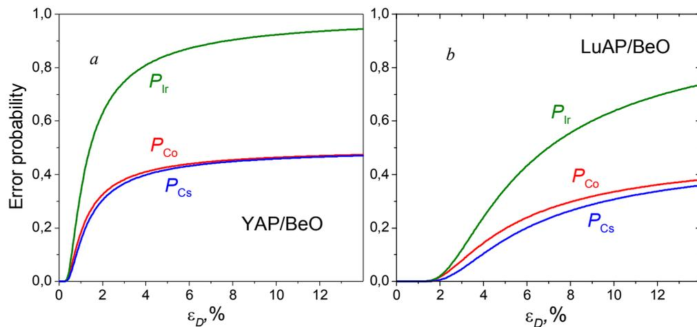
Fig. 4. Dependencies of the radioisotopes identification error probabilities  $P_{Co}$ ,  $P_{Ir}$  and  $P_{Cs}$  upon the relative error of the absorbed dose measurement  $\varepsilon_D$  according to the decision-making rule (6) and absorbed dose measurement using detectors pairs YAP/BeO (a) and LuAP/BeO (b)
