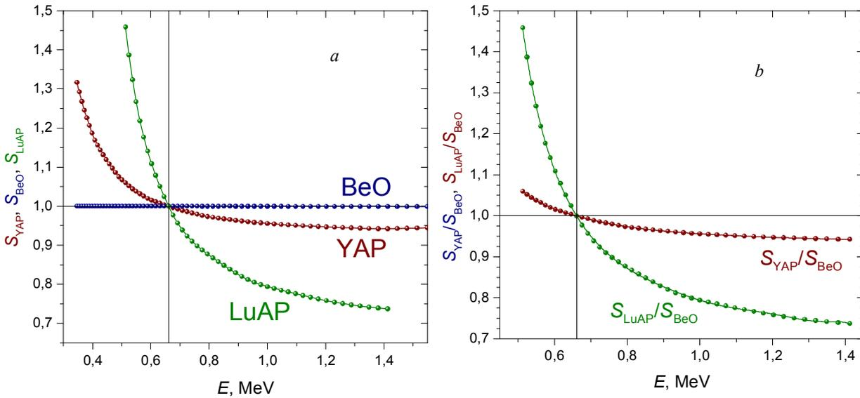
Fig. 2. Energy dependencies of relative sensitivity  $S(E)$  of the dosimetric detectors, based on YAP, LuAP and BeO (a) and their ratios  $R(E) = \frac{S_1(E)}{S_2(E)}$  (b) for heavy and light detectors
