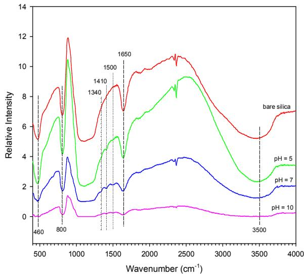
Fig. 4. FTIR spectra of glycine adsorbed on silica nanoparticles as a function of pH
