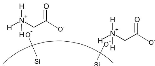
**Fig. 7.** Electrostatic interactions between glycine and silica surface at isoelectric point
