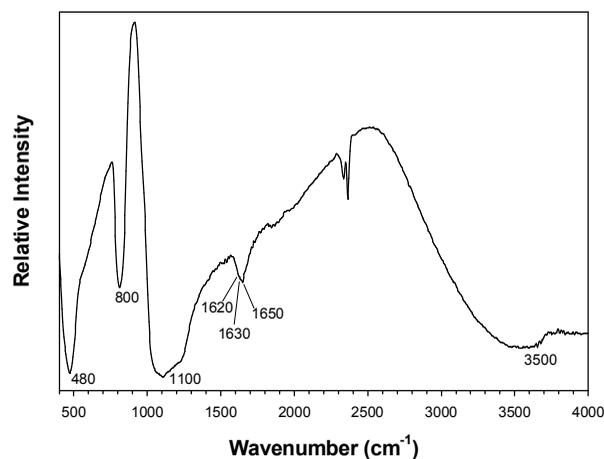
**Fig. 2.** The FTIR spectrum of silica nanoparticles synthesized using a microwave-assisted method
