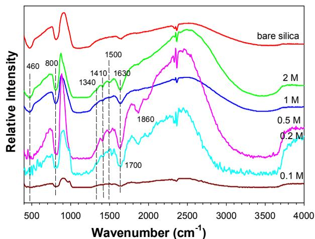
**Fig. 3.** FTIR spectra of glycine adsorbed on silica nanoparticles as a function of glycine concentration
