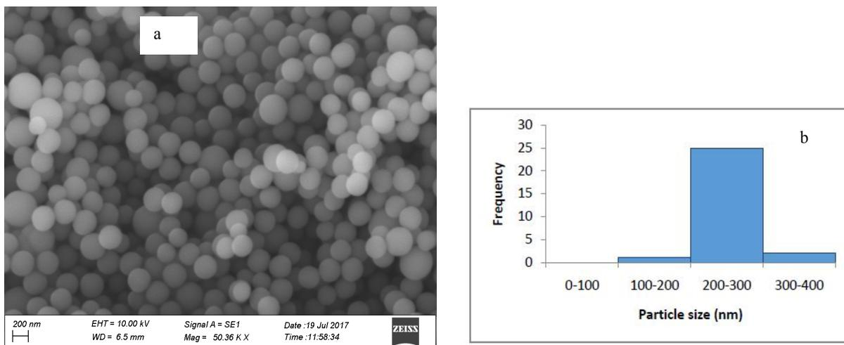
**Fig. 1.** SEM image of the silica nanoparticles synthesized using a microwave-assisted method (a). Particle diameter distribution for the synthesized nanoparticles (b)
