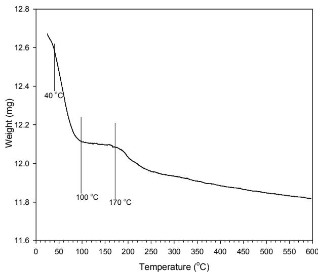
Fig. 5. Weight loss curve of glycine adsorbed on silica nanoparticles
