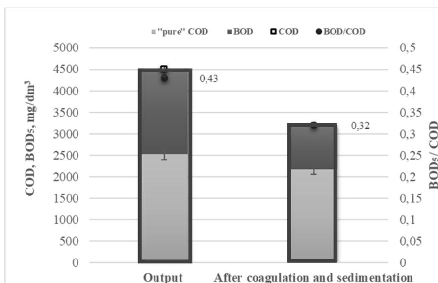
**Fig. 3.** Dynamics of organic matter concentration in terms of “pure” COD and BOD<sub>5</sub> for the initial industrial wastewater and after its coagulation
