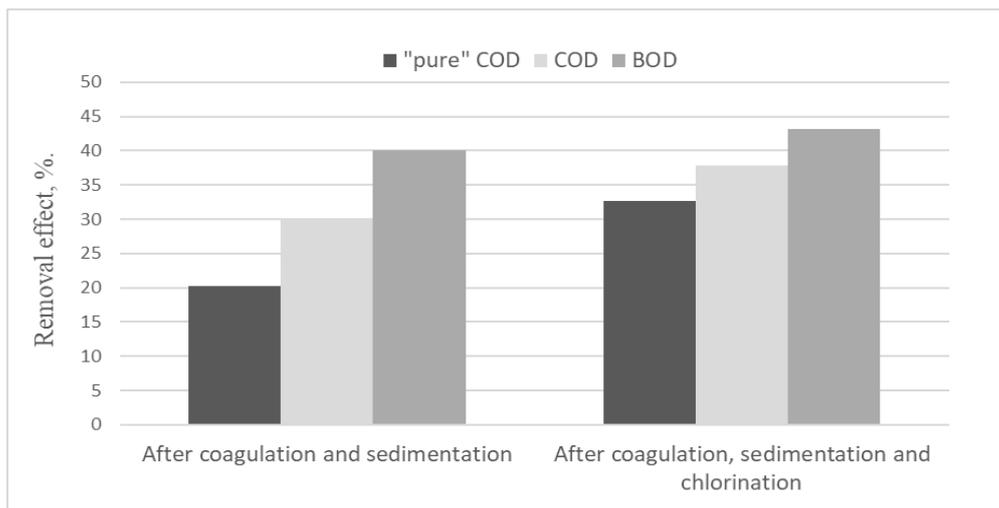
Fig. 2. Comparison of the effect of organic matter removal in terms of "pure" COD, BOD<sub>5</sub> and COD after coagulation and after coagulation and chlorination
