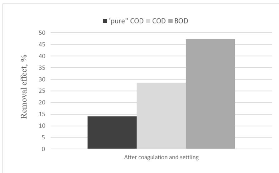
**Fig. 4.** Effect of organic matter removal in terms of “pure” COD, BOD<sub>5</sub> and COD after coagulation and settling of industrial wastewater
