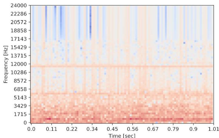
**Fig. 7.** Spectrum plot of screw press work with seeds.
