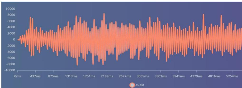
**Fig. 3.** Waveform of screw press work with seeds.
