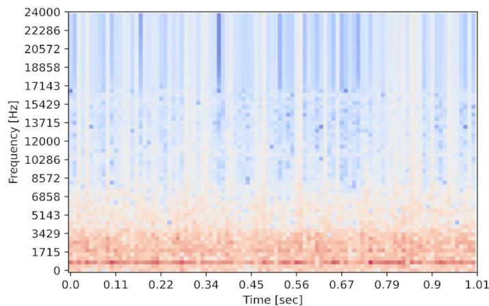
**Fig. 6.** Spectrum plot of screw press work without seeds.
