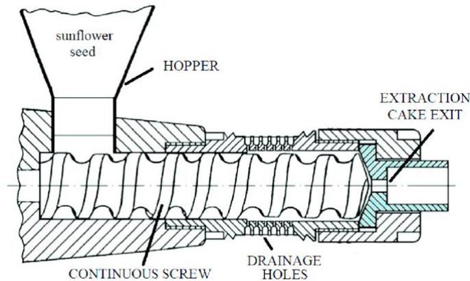
**Fig. 1.** Oil screw press [2]
