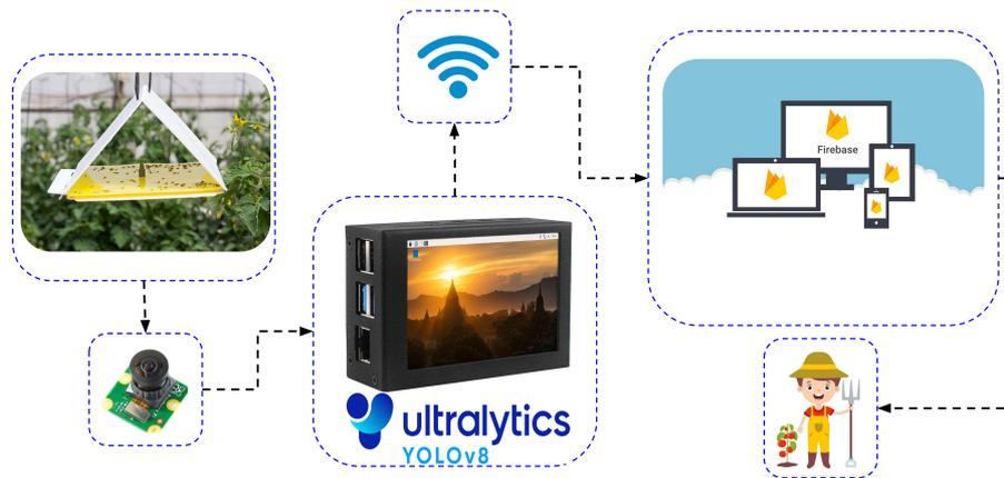
Fig. 7. Structural design of a device for pest counting.
