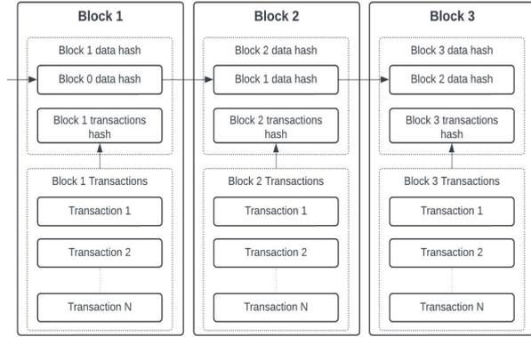
Fig. 1. Chain of blocks in a blockchain
