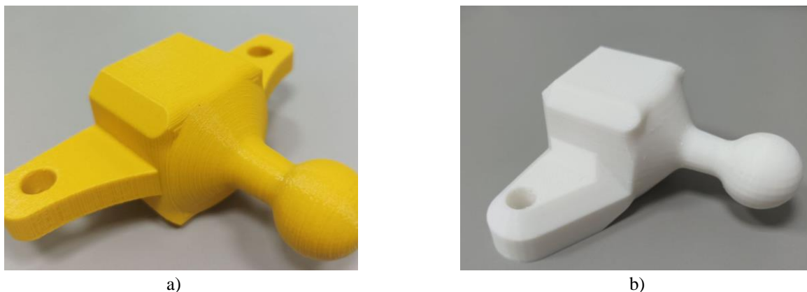
Fig. 3. a) The part is printed on coPET, humidity - 40%.; b) The part is printed in PLA, humidity - 44%.
