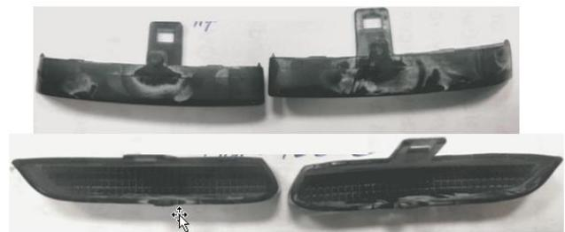
**Fig. 12.** The general view of the parts from PA12 with increased injection speed and changed cooling temperature of the injection molding tool after aging in  $C_2H_5OH$  96.6 vol.%
