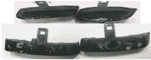
**Fig. 9.** General appearance of the PA12 product with increased injection speed after aging in C<sub>2</sub>H<sub>5</sub>OH 96.6 vol.%
