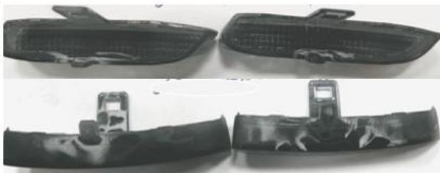
Fig. 5. The general view of the product from PA12 using standard process parameters after aging in  $C_2H_5OH$  96.6 vol.%
