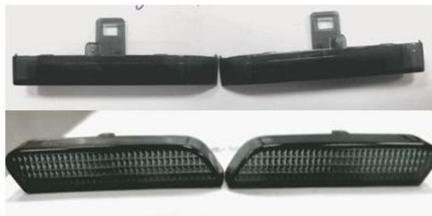
**Fig. 2.** General view of the parts obtained from PA12
